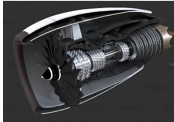
Figure 3. Turbofan jet engine [7].
