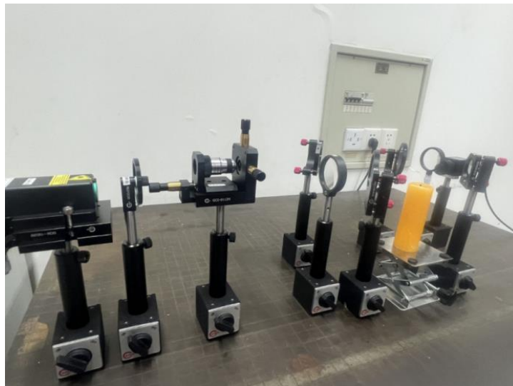
Figure 3. Mach-Zehnder optical path
