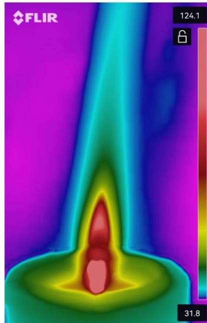
Figure 6. Infrared measurement of the candle temperature
