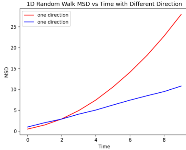
Figure 1. Comparison of MSD of different directions. The blue line is the regular result of MSD change with time. According to Einstein's Relationship, the blue line can be approximated seen as a linear relationship, which the slope would be six times the diffusion coefficient. The red line is the result when particles could only move towards one direction, which indicates MSD and time have a quadratic function relationship.
