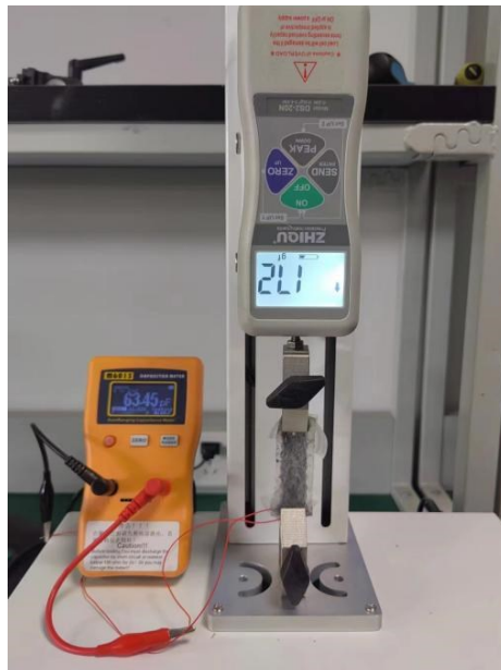
Figure 12. Basic tensile test setup
